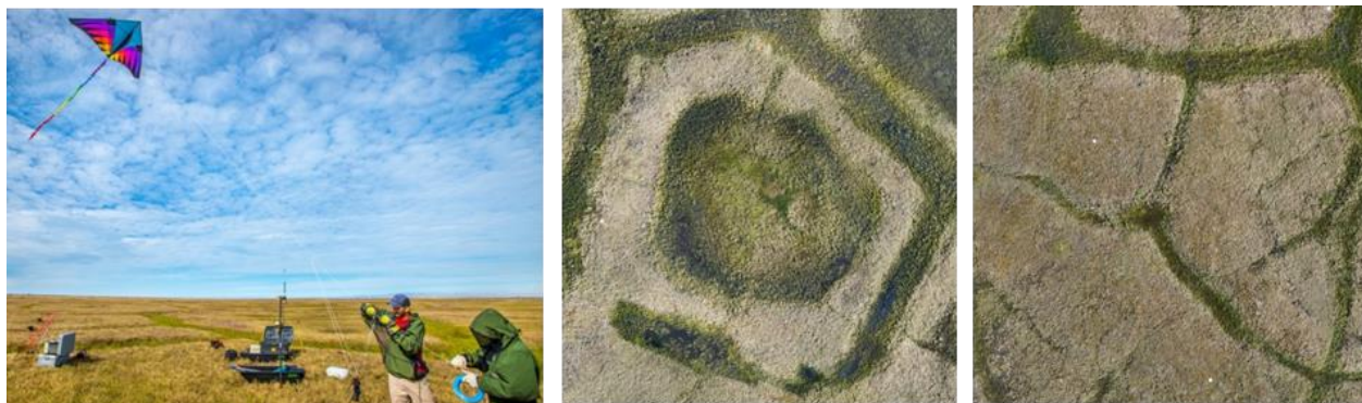
The picture on the left shows the co-acquisition of electrical resistivity tomography (ERT) along transects on the Barrow Environmental Observatory. Geophysical data acquired using the ERT arrays are collocated with point-scale measurements of various soil properties and landscape images using a kite-based platform equipped with a multi-spectral camera. Landscape images (such as the ones shown on the right) are involved in the reconstruction of geo-referenced mosaic and digital surface model, which are further used to investigate co-interactions between subsurface and surface properties.
